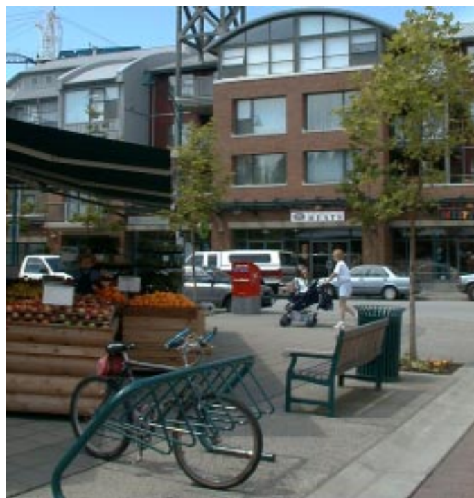
Bicycle parking should be incorporated into the design of sites and designed to be an integrated feature of the streetscape (rather than being seen as an element that looks “tacked on”)
