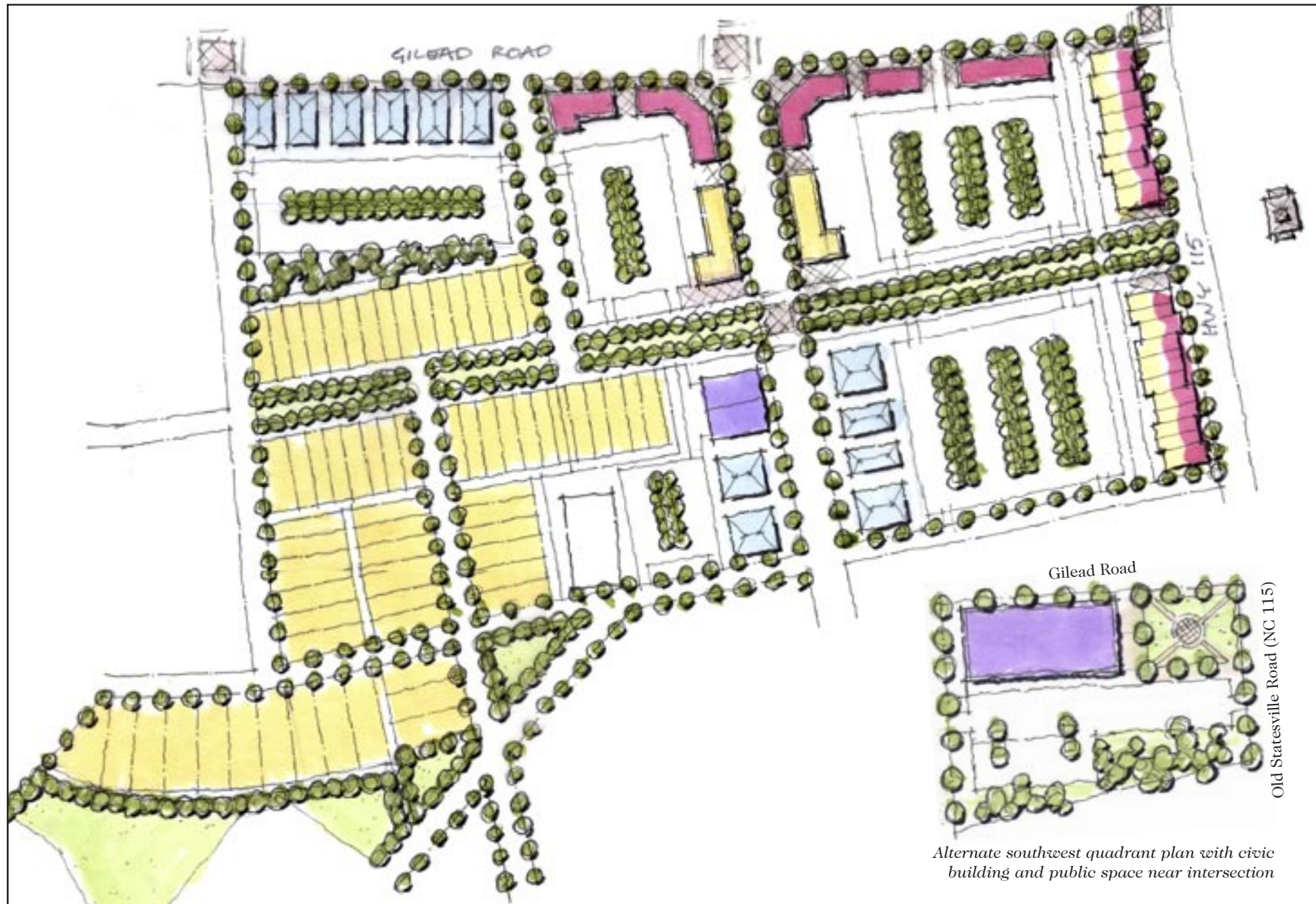
Alternate Plan for the southern quadrants with Single Family, Offices, and Mixed-Use Buildings and a grand public green space running east to west
