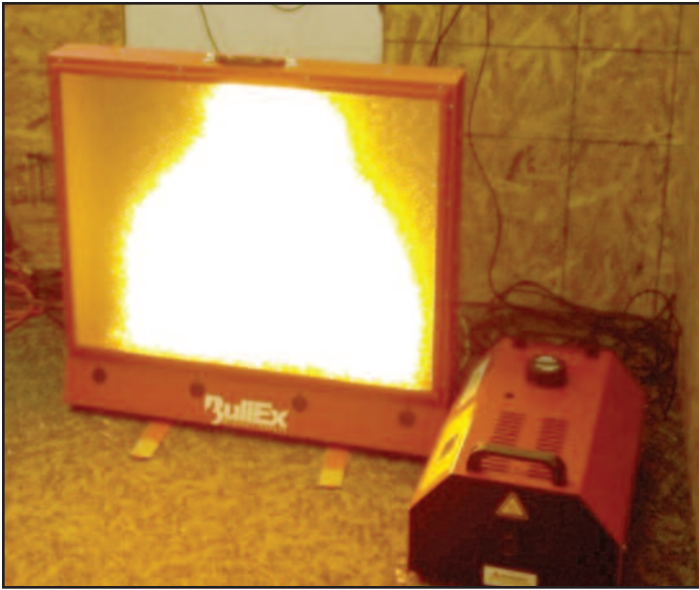
Figure 4: Fire display and smoke generator
