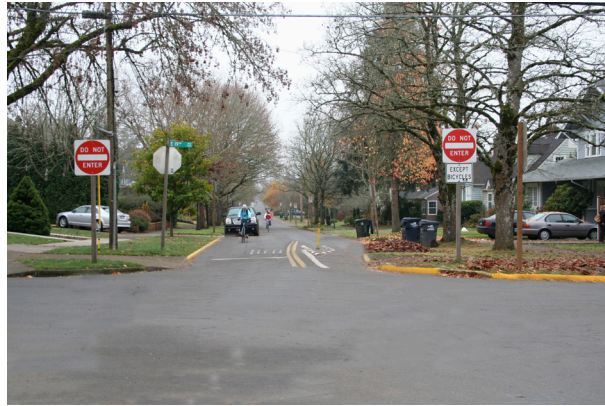
Figure 35: Pinch point at F Street intended to divert motorized traffic away from the entrance of the bike boulevard.
