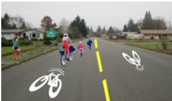
Figure 10: Sharrows on Pheasant Street.
