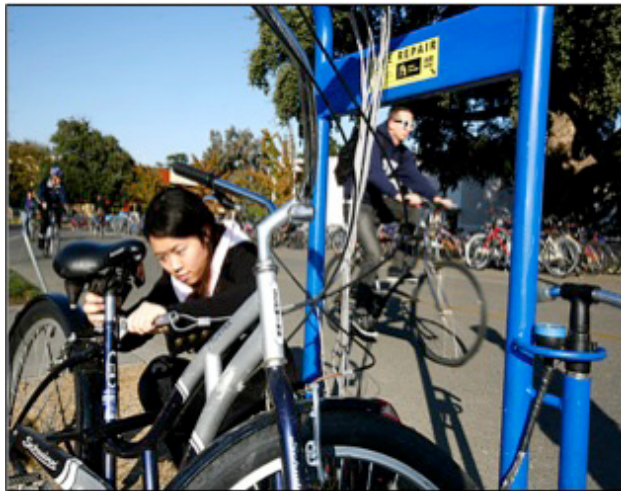
Figure 23: This is an example of a bike maintenance rack that might be installed at the park and ride area. It includes bike maintenance tools as well as an air pump for bicyclists using the path. (Image courtesy of davisenterprise.com.)
