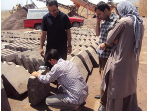
Herat construction staff practice using the digital concrete hammer
