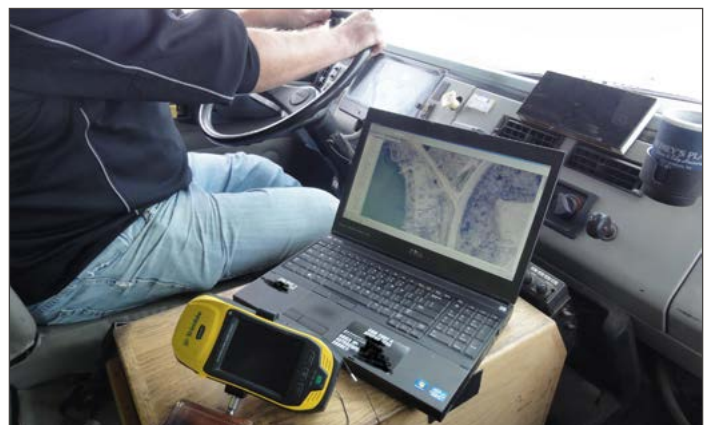
Field crews can enter locational data directly into the county's GIS system while in the field rather than having to wait until they return to the office.
