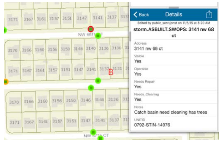
Fort Lauderdale's SWOPS application, which is used to carry out the NPDES stormwater activity mandated by the State Department of Environmental Protection, saves numerous labor hours.
